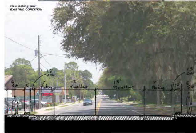
Existing Pennsylvania Avenue Typical Section
