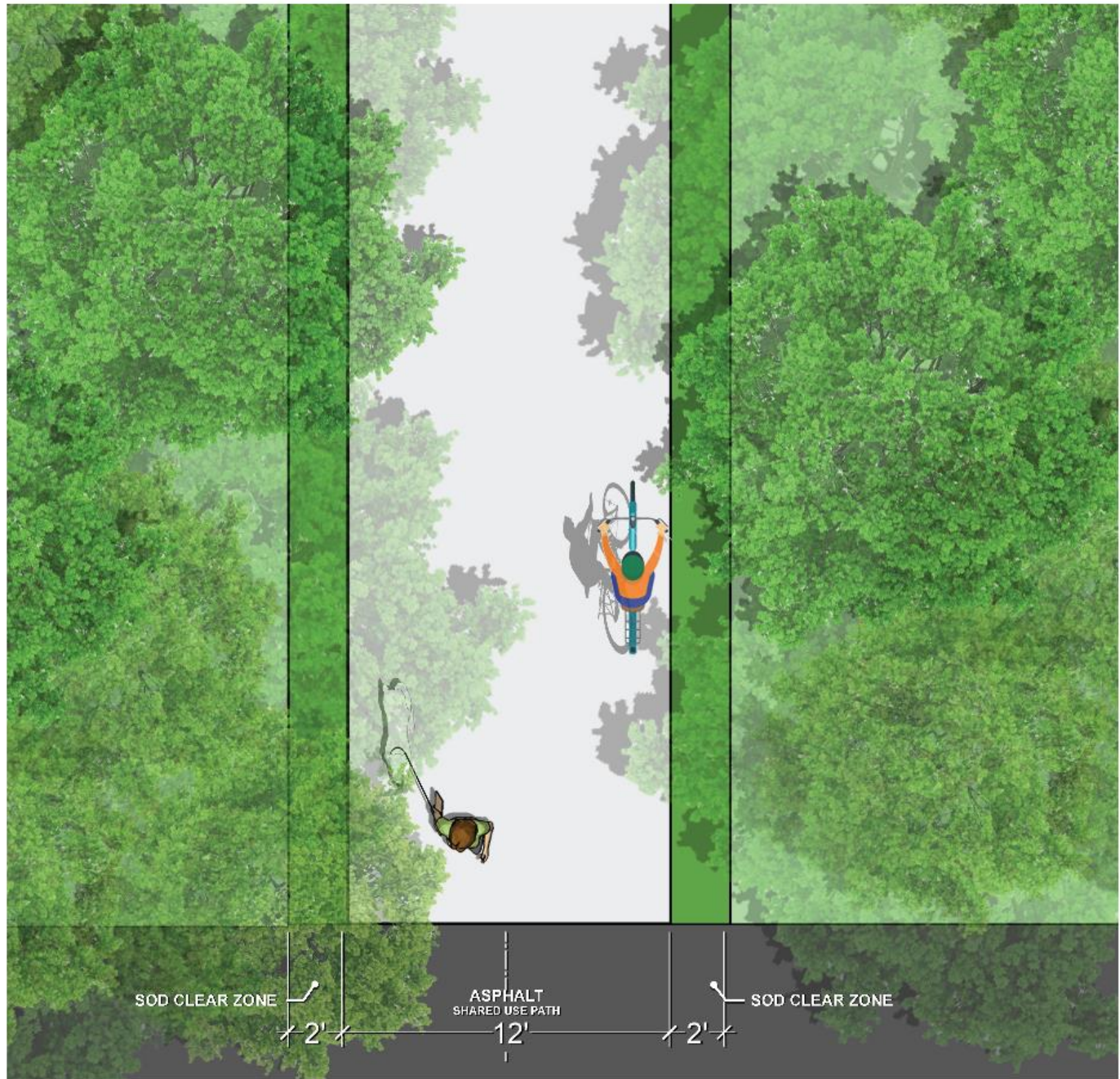
Paved Trail: Typically 10-12 ft. wide asphalt with a 2 ft. clear zone on each side.
