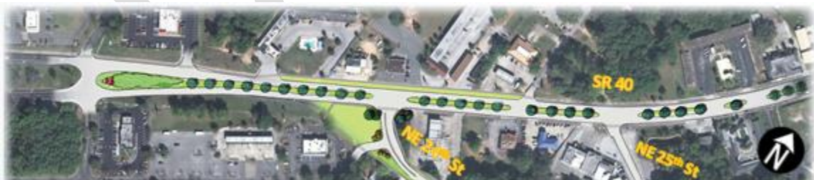
Figure 21: NE 24 th Street and NE 25 th Street Realignment – No Turn Lanes
