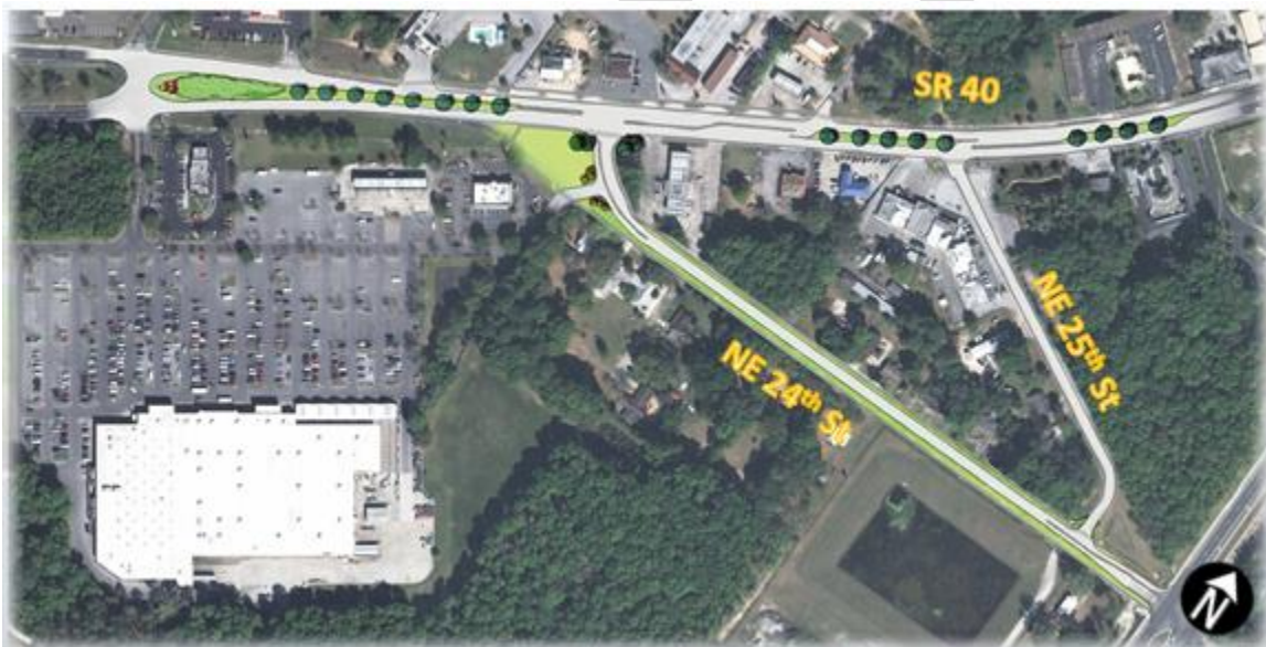
Figure 20: NE 24 th Street and NE 25 th Street Realignment – With Turn Lanes
