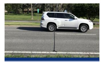
The majority of all count stations in Marion County are temporary count stations. These sites feature a portable count computer and pneumatic tubes that are taped across the roadway. When driven over, a burst of air pressure is sent through the tube to the counter. For each vehicle that passes over the tubes, the counter records the time of occurrence. **Permanent Stations**
