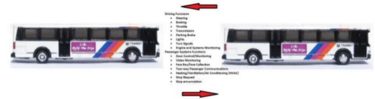
Schematic – Wireless Short-Range Connections Between Buses Interface with Automated Driving and Passenger Systems Functions
