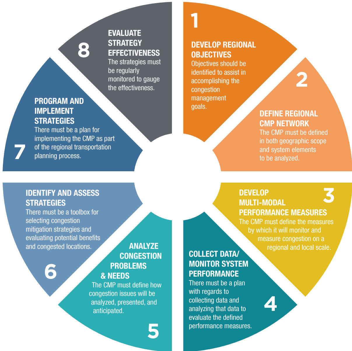
Figure 3: Federal Eight-Step Congestion Management Process
