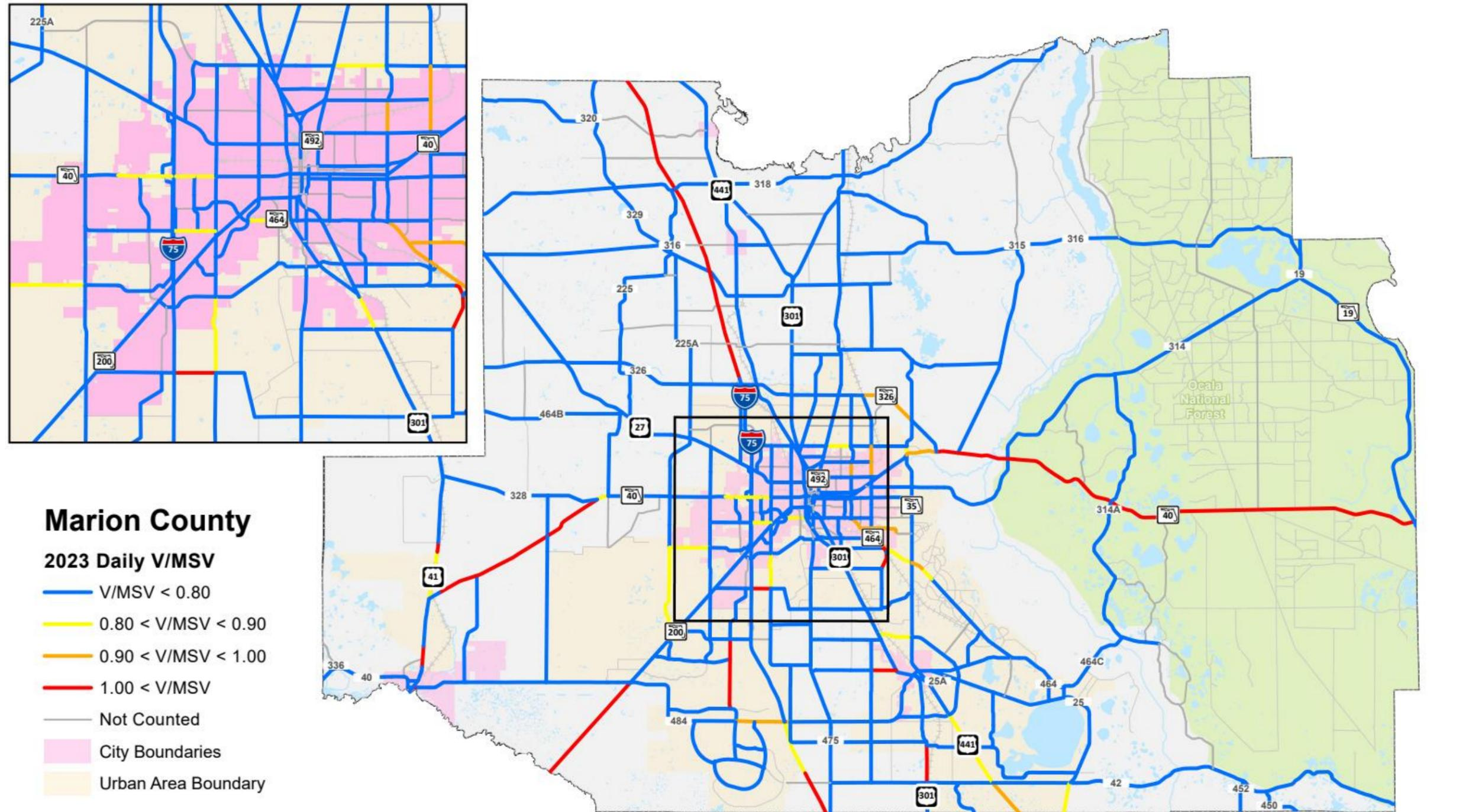
Volume-to-MSV ratios are calculated as the daily volume divided by the maximum service volume of the roadway segment based on its adopted level of service standard.
